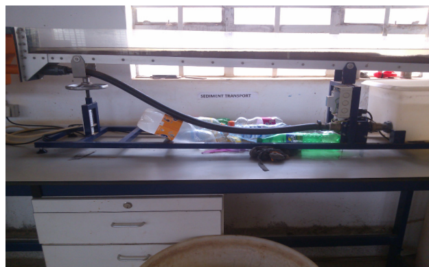
Figure 1; 1.2m long circulating flume simulating sediment transport
