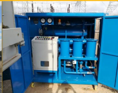
9000l/hr Oil Filtration Machine with 2140 m3/hr Double Stage Vacuum Pump
