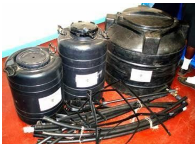
Different sizes of a simple gravity fed drip irrigation system showing the other accessories (including the drip pipes).
