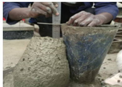
Figure 4. Slump test on fresh concrete.
