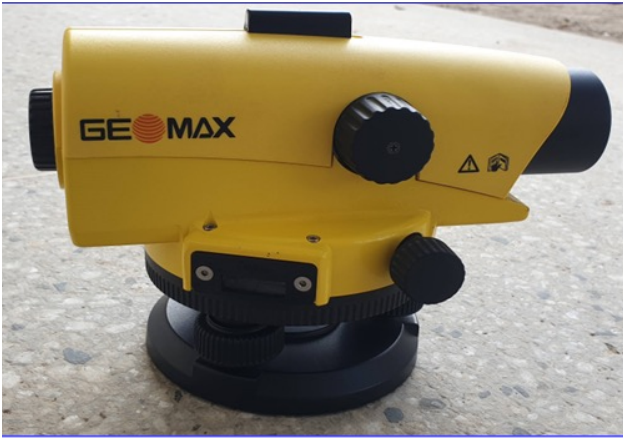
Automatic level: H, slope measurements
