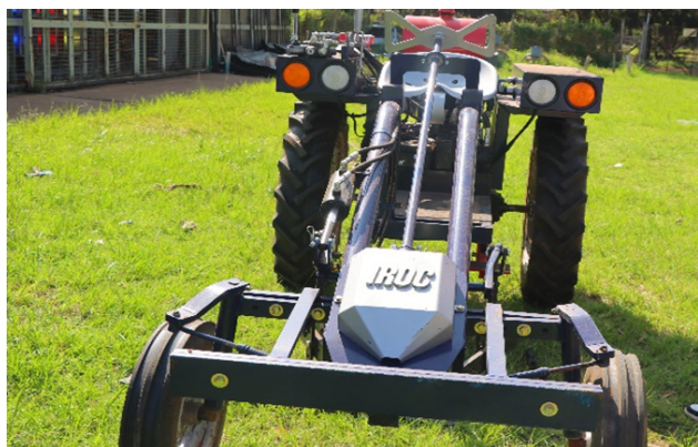
The IROC Tractor (20 HP), an innovative creation from JKUAT, is powered by petrol and is generally fuel-efficient with reduced emission potential, thus significantly reducing CO 2 emissions. This eco-friendly design enhances climate resilience by promoting sustainable agricultural practices for smallholder farmers.
