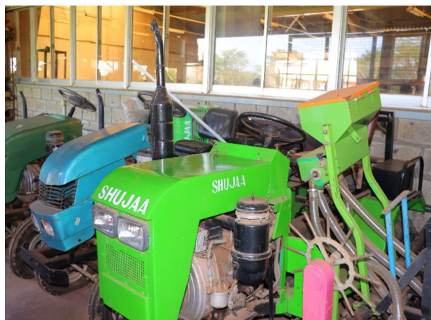
The Shujaa Tractor, an innovative solution from JKUAT, has a power rating of 10.5 HP (to be upgraded to 16 HP) and is designed to revolutionize agricultural mechanization for smallholder farmers. Engineered for near-zero environmental impact, it combines efficiency and sustainability, setting new standards in green farming technology.
