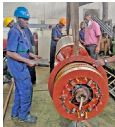
3 Megawatts turbine generator rotor after servicing ready to be installed in the main stator.
