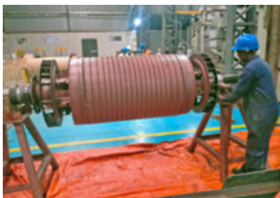
Confirmation of the bearing journals for the right tolerance on the slipring rotor.
