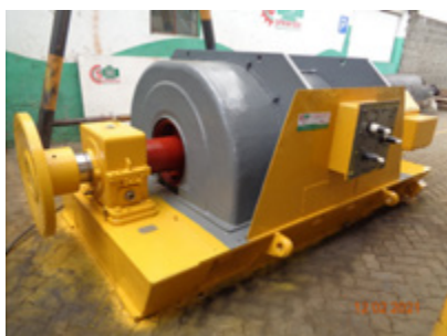
1600 kW slipring motor after comprehensive refurbishment.
