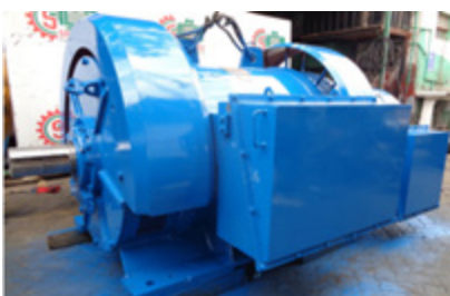
930 kW Slip Ring motor, Completely Rewound Rotor winding using imported bar winding materials to class H insulation.
