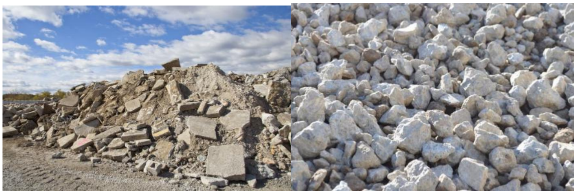
Figure 3.1: Disposed Demolitions and Recycled aggregates
